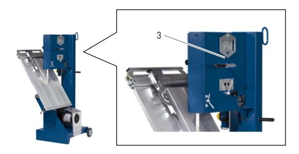
• Lubricate the automatic power chuck above the opening (Pos. 3) on the tensioning lever with a spray oil
